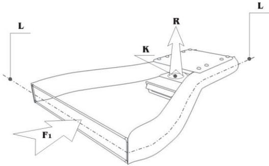
by towing or by using its own drive. The device is constituted by a funnel-shaped collector plate tapered from the larger cross-section, in the direction of motion, to the lower section, in the queue according to the motion. It is equipped with a front opening and with one or more rear openings.
