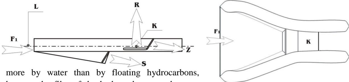
more by water than by floating hydrocarbons, because the film of the hydrocarbons can be very thin and for the effect of water motion. The openings controlled on the face of the funnel immersed allow the escape of the excess water, in order to convey the maximum possible rate of hydrocarbons into the suction area of the pump (K in figure 2).
